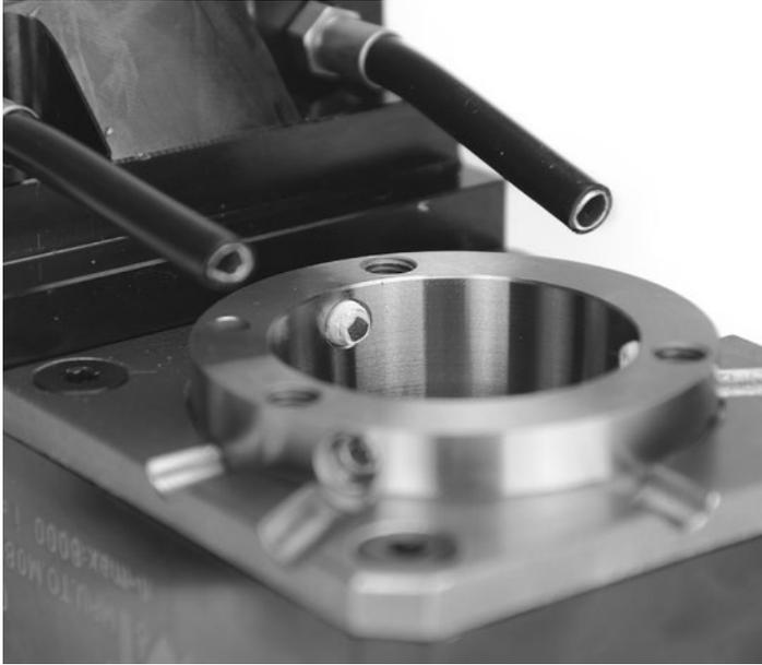
By the use of the modular thread whirling head, the mounting and dismounting of the unit out of the machine and the steady adjustment, are now things of the past. Though the high rotation accuracy of the interface and the even wear of the cutting edges, tool endurance can be increased up to 300%.
